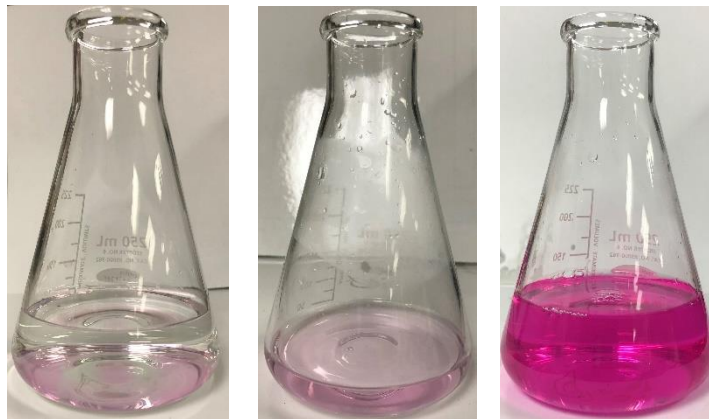
Figure 2: Three samples show titrations (1) before endpoint (2) at endpoint and (3) past endpoint
