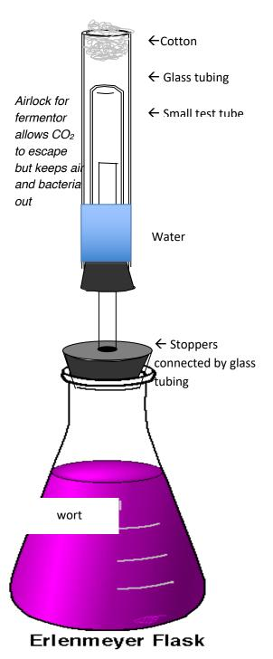
air lock consists of a large glass tube containing an inverted test tube, water at the bottom, and a cotton plug at the top.
