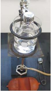
**7**) Accurately measure the volume of the flask (it is more than 125 mL!) by filling it with water all the way to the brim and measuring the volume of water with a 100 mL graduated cylinder. Record the flask volume on the report form.
