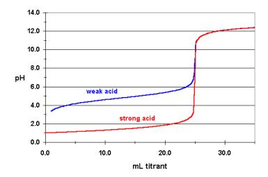
The titration curve for the addition of a base to a strong acid and for the addition of a base to a weak acid. The area of the graph where the pH is not significantly changing (between 0.0 mL and 20 mL in this example) is called the buffer region.
